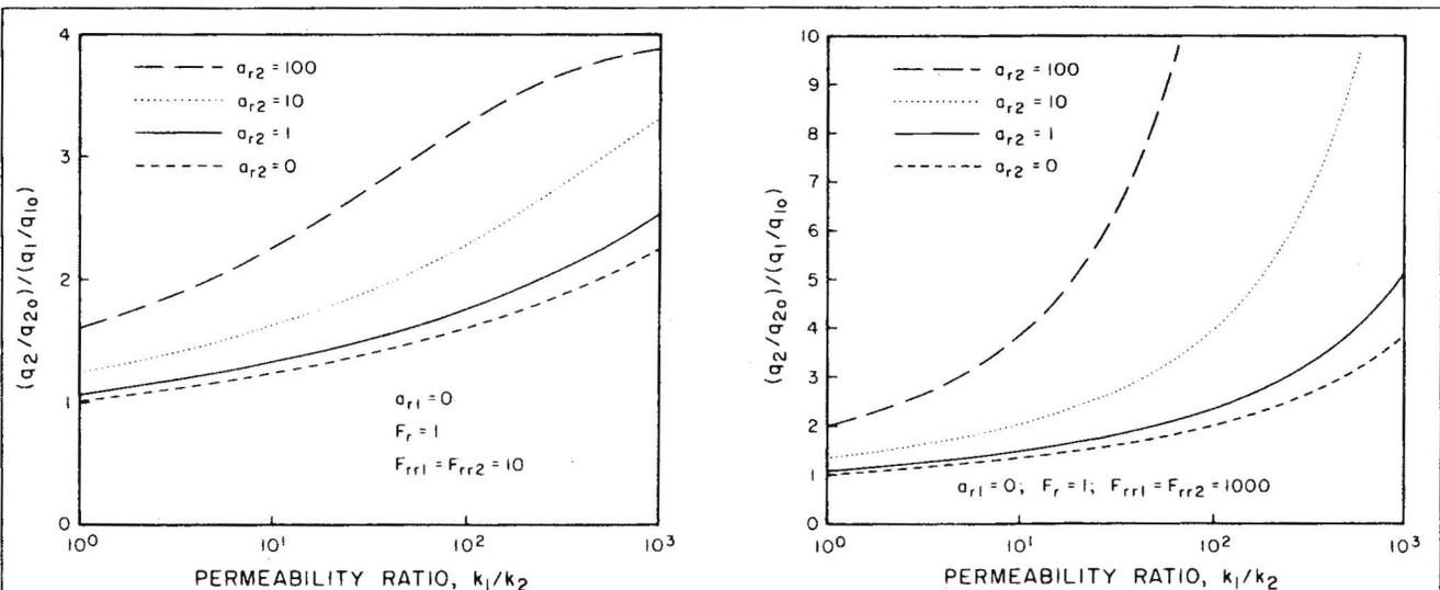
Fig. 8—Best-case profile improvement in radial flow: (a) weak gel ( $F_{rr} = 10$ ) and (b) strong gel ( $F_{rr} = 1,000$ ).
