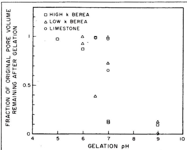
Fig. 5—PV remaining after gelation vs. gelation pH.
